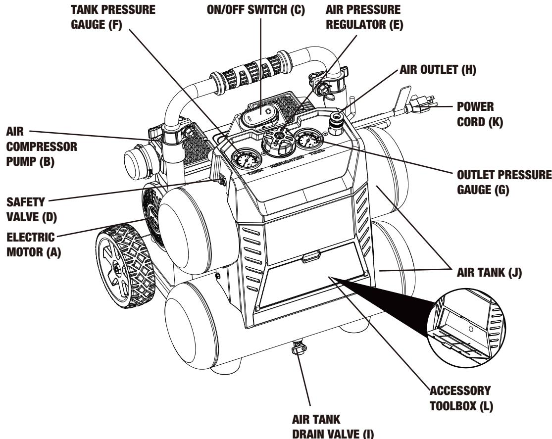
**A. ELECTRIC MOTOR:** The motor is used to power the pump. It is equipped with a thermal overload protector. If the motor overheats for any reason, the thermal overload protector will shut it down in order to prevent the motor from being damaged.
