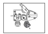
3.5. Pull the drive roller off of the drive roller shaft.
