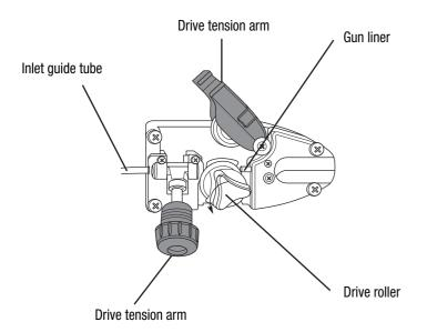
3.1. Open the door to the welder drive compartment.
