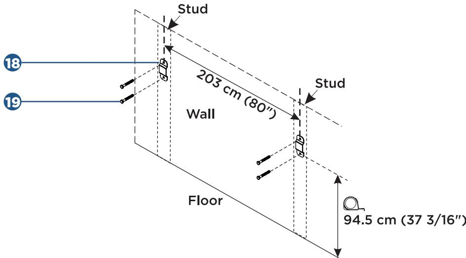
Install another two safety brackets (18) to both sides of the cabinet with four M6 x 12 hex bolts (2). Tighten securely.
