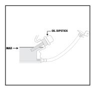
4 Check engine oil level at every use and add as needed.
