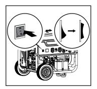
Press and hold the ignition switch to the "START" position. Release as the engine begins to start. If the engine fails to start within five seconds. release the switch and wait at least 10 seconds before attempting to start the engine again.
