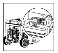
Do not over-choke. As soon as engine starts, move the choke to the "RUN" position over a 2–5 second duration.
