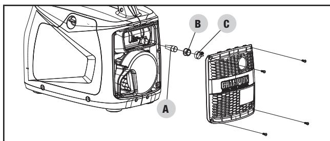
4. Remove the spark arrestor screen.
