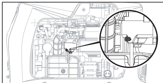
6. When gasoline stops flowing from the clear tube, rotate drain screw clockwise until tight. Properly dispose of the drained gasoline according to local regulations or guidelines.
