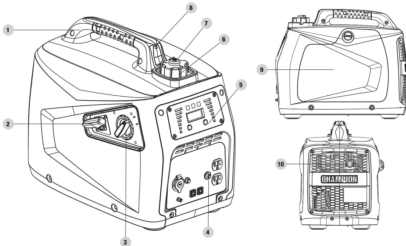
1. **Carrying Handle** – Used to lift or carry the unit.
