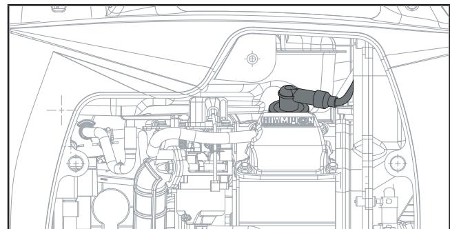
2. Remove the spark plug wire from the spark plug.
