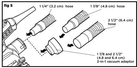
When the dust canister is removed from the tool, a vacuum hose accessory (available separately) can be attached to the dust port. To use this feature, attach the vacuum hose to the dust port, then connect the opposite end of the vacuum hose to a shop vacuum cleaner. A 2-in-1 vacuum adaptor is included for connection of this tool to a 1 7/8 or 2 1/2" (4.8 or 6.4 cm) vacuum hose. A 1 1/4" (3.2 cm) vacuum hose may be connected directly to the tool without an adaptor.
