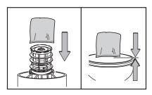
8 For wet vacuum cleaning, remove the reusable cloth filter, and install the supplied foam wet filter. See page 22 for the foam wet filter installation instructions.
