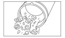
Clear all dirt or debris from the collection tank and hose into a proper waste container.
