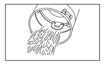
After use, empty the collection tank, clean, and dry the inside and outside of the collection tank.
