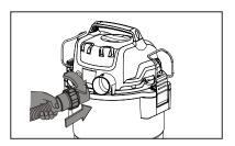
2 Make sure the collection tank is empty before using it as a blower. Clear all dirt and debris from the hose and collection tank. Remove the hose from the vacuum port. Insert the locking end of the hose into the blower port on the back of the powerhead and lock it into place.
