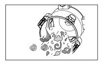
4 Clear all dirt or debris from the collection tank and hose into a proper waste container.
