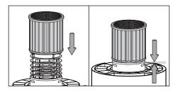
2 Remove the powerhead and place in an upside-down position. Install the cartridge filter over the filter cage making sure the cage is completely covered.
