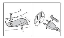
Verify that the switch is in the 'O' OFF position before plugging the power cord into the power outlet. Plug the power cord into the outlet.
