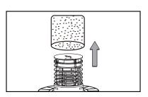
With the removed powerhead in an upside-down position, carefully remove the foam wet filter.
