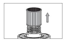
With the removed powerhead in an upside-down position, carefully remove the cartridge filter from the filter cage.
