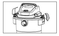
3 Lift the powerhead off the collection tank.
