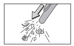
6 The unit will now blow through the vacuum hose and can be used to clear obstructions within the hose.
