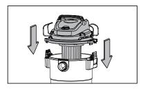
Place the powerhead back on the collection tank and secure it in place using the latches.
