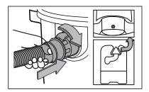
10 Insert the locking end of the hose into the port on the collection tank and turn to lock into place.
