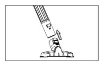
6 The included accessories lock together to prevent them from detaching during use. Connect the desired accessory onto the end of the hose or extension wand by aligning the tabs and push together until they lock into place.
