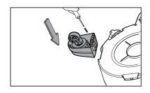
6 Position the left hose storage rack on the front side of the powerhead, just above the top edge of the tank, as illustrated. Squeeze the open sides of the left hose storage rack inward and insert the open ends into the allocated slot. Verify that the rack is secured in place. Install the right hose storage rack in the same way on the other side of the powerhead, ensuring it is secured.
