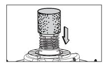
8 For wet vacuum cleaning, remove the cartridge filter, and install the supplied foam wet filter. See page 24 for the foam wet filter installation instructions. 9 Place the powerhead back on the collection tank and secure into place using the latches.
