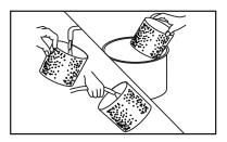
3 Allow the wet filter to air dry completely before storing or installing onto the filter cage.
