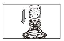
8 For wet vacuum cleaning, remove the cartridge filter and install the supplied foam wet filter. See page 21 for the foam wet filter installation instructions.
