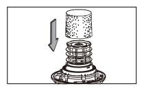
Carefully slide the foam wet filter down over the filter cage making sure the cage is completely covered. Place the power head onto the collection tank.
