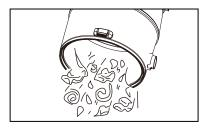
4 Clear all dirt or debris from the collection tank and hose into a proper waste container.
