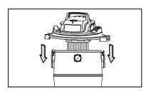
Place the power head back on the collection tank and secure it in place using the latches.
