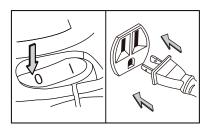
Verify that the switch is in the '0' OFF position before plugging the power cord into the power outlet. Plug the power cord into the outlet.
