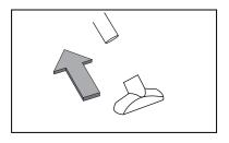
6 Push the required attachment onto the free end of the hose or extension wand.
