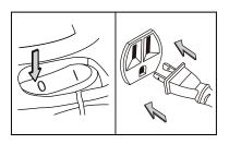
Verify that the power switch is in the '0' OFF position before plugging the power cord into the outlet. Plug the power cord into the outlet.
