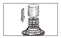
2 Remove the cartridge filter, then carefully install the foam wet filter over the filter cage and place the power head back on the collection tank. For foam wet filter installation instructions, see page 21.
