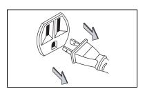
Once you have completed vacuuming, flip the switch to the 'O' OFF position. Unplug the power cord from the outlet.
