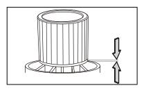
In order to prepare your vacuum for dry vacuuming, make sure the cartridge filter completely covers the filter cage against the power head. Your wet/dry vacuum comes with the cartridge filter pre-installed. For installation instructions, see page 20.
