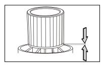
2 Remove the power head and place in an upside down position. Install the cartridge filter over the filter cage making sure the cage is completely covered.
