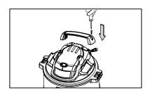
6 Insert the handle into the slots located on the top of the power head and secure it with the screws provided. Do not over-tighten the screws.
