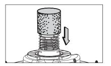
2 Remove the cartridge filter and install a foam filter over the filter basket and place the top section back on the tank. DO NOT USE THE CARTRIDGE FILTER FOR LIQUID VACUUMING.
