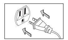
4 Ensure that the switch is in the "O" (OFF) position before plugging the power cord into the power outlet.
