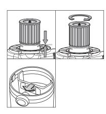
8 For wet vacuum cleaning, install the supplied foam filter.
