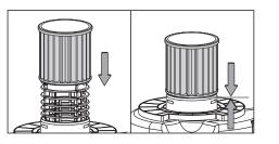
2 Place retainer on top of cartridge filter against hole of basket.
