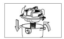
4 Insert the locking end of the hose into the vacuum port and lock in place.
