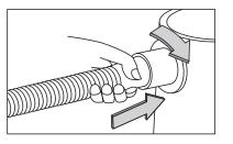
12 Choose the desired accessory and insert onto the end of the hose.
