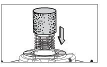
Replace the top section on the tank.
