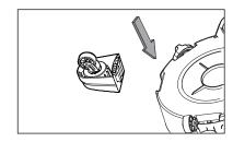
6 Position the hose storage rack as illustrated. Fully insert one end of the hose storage rack into the slot illustrated buy the arrow, then pull the other end of the hose storage rack to insert into the slot until it is secured in
