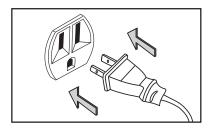
4 Ensure that the switch is in the "O" position before plugging the power cord into the power outlet.
