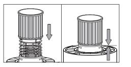
Place retainer on top of cartridge filter against hole of basket.
