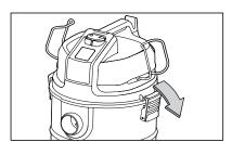
3 Lift the top section off the tank.
