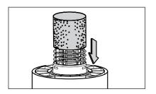
2 Remove the cartridge filter and install a foam filter over the filter basket and place the top section back on the tank.
