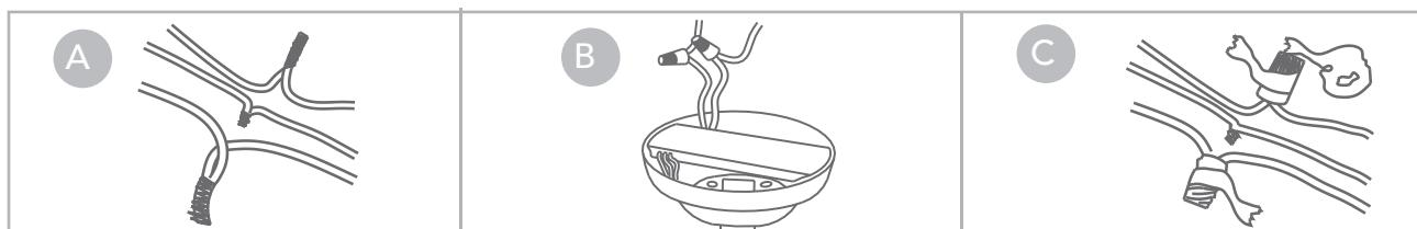
**⚠ WARNING:** Secure the connectors with electrical tape and ensure there are no loose strands or connections.
