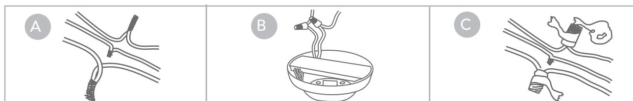
**⚠ WARNING:** Secure the connectors with electrical tape and ensure there are no loose strands or connections.
