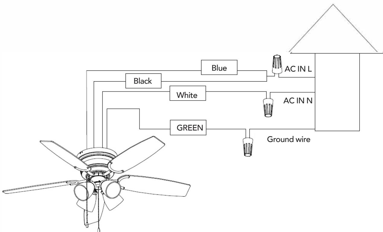
When wires are matched up, connect them by twisting frayed ends together (see Fig. A). Screw wire connectors (3 are provided) onto the tops of the twisted wires (see Fig. B). Fasten them with electrical tape (see Fig. C).
