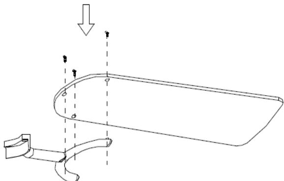
Install the blade arms with blades on the main assembly (see Fig.7B).
