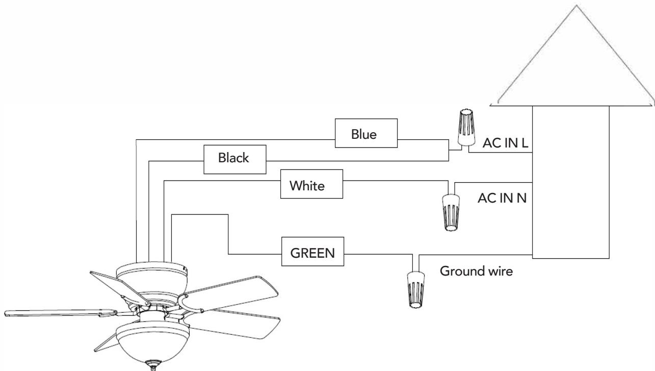
When wires are matched up, connect them by twisting frayed ends together (see Fig. A). Screw wire connectors (3 are provided) onto the tops of the twisted wires (see Fig. B). Fasten them with electrical tape (see Fig. C).
