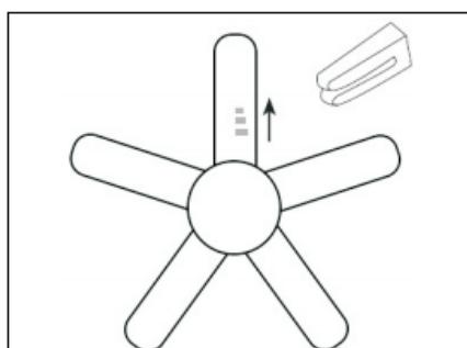
• Place the clip on the blade that needs the counterweight and place in different locations, from the centre to the tip of the blade, until the wobble disappears.
