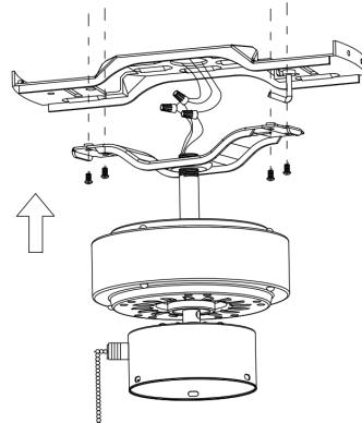
**Note:** Attach safety cable from fan unit to "J" hook in outlet box. Secure by looping zip tie through safety cable and "J" hook. Tighten zip tie securely.
