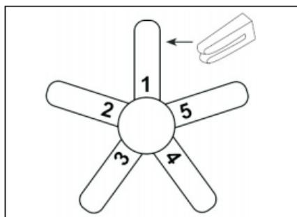
• Put the clip on the centre of a blade. Turn on the fan and if the wobble persists, put the clip on another blade until the wobble is reduced. Replace the balancing clip with counterweight provided in the balancing pieces.
