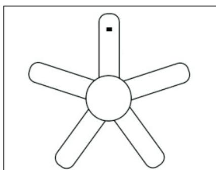
• Paste the counterweight on the surface of the blade near the clip, remove the clip and test the fan. If vibrations persist, put on another counterweight. If it gets worse, try another area to place the weight.
