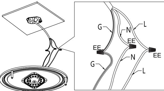
3. Connect the black wire(s) from the fixture to the black (live) wire of the supply circuit and screw on a wire connector.
