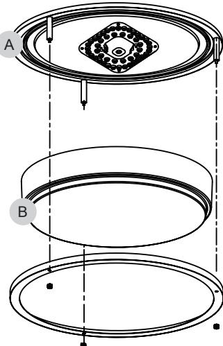
7. Add the light shade (B) to the fixture pan. Add top ring over light shade and use the 3 hold-down nuts (included with light shade) to secure ring.
