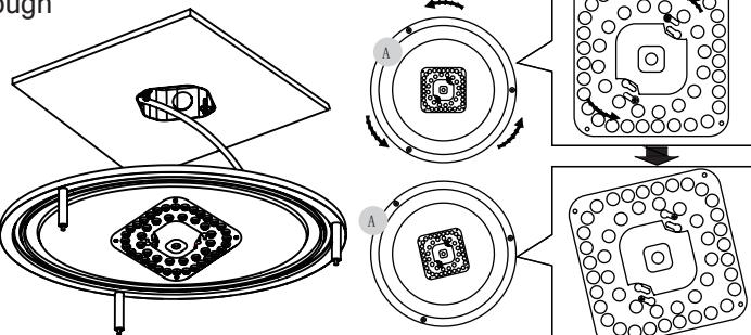
6. Tighten the mounting screws so that the fixture pan is secured flush with the ceiling.
