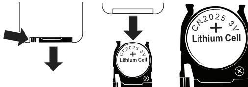
The battery used in the remote control is a CR2025 button cell. When the battery needs to be replaced, open the battery tray by pushing in on the tray tab and pulling the tray out. The tray is marked with a "+". Install the battery to match (with the "+" up).
