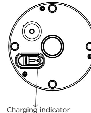
If the battery can't be charged or if fully charged but does not work as before, replace the battery. Remove screws and replace with same type rechargeable battery (3.7 V 18650, 2000 mAh). See image below.
