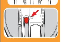
9. Open the SnugLock® Lock-Off Lift the lever to open the SnugLock® lock-off.
