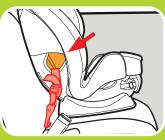
6. Make Sure UAS Strap is in the Forward-Facing Belt Path Marked with Orange Label
