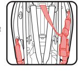
If the UAS strap interferes with the vehicle seat belts or if the chosen seating position does not have lower anchors, you MUST store the UAS connectors. Store the UAS connectors by attaching to the plastic bars as shown. Store the top tether as shown. Always secure car seat with UAS or a vehicle seat belt, even when unoccupied. In a crash, an unsecured car seat can injure passengers.
