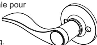
3. Tighten the screw by hex key to complete the lever handing changing.
