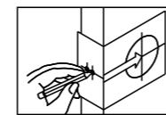
Select 60 mm or 70 mm (2 3/8" or 2 3/4") backset as desired and mark centre of hole on door face.
