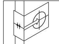
Backset is the distance from door edge to centre of hole on door face. Some locks are supplied with an adjustable latch that can fit 60 mm (2 3/8") or 70 mm (2 3/4") backset. Follow the steps shown below to change backset.
