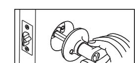
Install inside lever and tighten screws until lock is tight.
