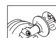
Insert spindle through latch. Press flush against door.
