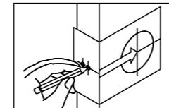
Select 60 mm or 70 mm (2 3/8" or 2 3/4") backset as desired and mark centre of hole on door face.
