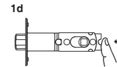
To reset the latch to 60 mm (2 3/8") backset, push spindle cam to the left end of the adjusting hole.
