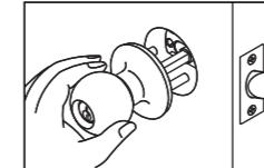
Insert spindle through latch. Press flush against door. Note: Key hole must be in down position.
