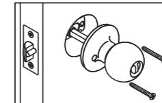
Install inside knob and tighten screws until lock is firm.
