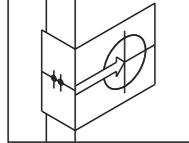
Backset is the distance from door edge to centre of hole on door face. Some locks are supplied with adjustable latch which can fit 60 mm (2 3/8") or 70 mm (2 3/4") backset. Follow the steps shown below to change backset.
