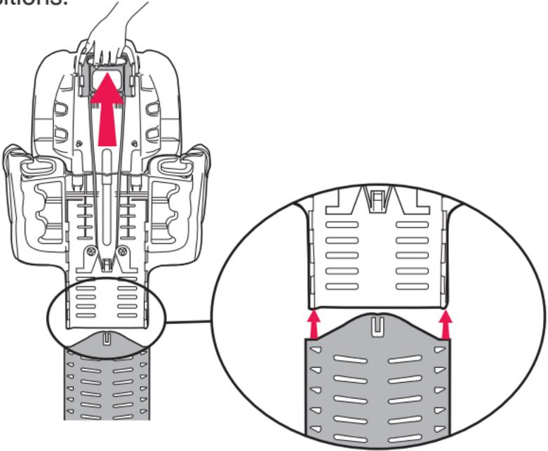
4. **Attach the seat pad to the backrest assembly.**
