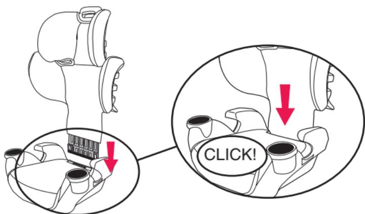
7. **Check your work.** Inspect the Booster Seat. Pull up on the headrest to make sure it is securely attached to the backrest. Make sure the seat pad is hooked into place. Pull on the backrest to make sure it is securely attached to the base. Repeat any assembly steps as necessary.
