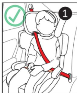
**! WARNING:** You **MUST** use the vehicle 3-point lap-and-shoulder belt when restraining the child in the booster seat **1**. UAS **WILL NOT** secure your child in the booster seat.
