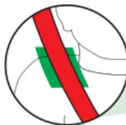
3. Thread both sides of the lap belt under BOTH armrests. Thread the lower end of the shoulder belt under the armrest on the buckle side ①.
