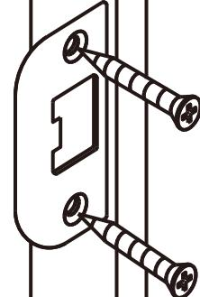
Install strike and tighten screws.
