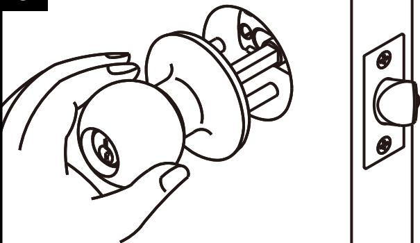
Insert spindle through latch.
