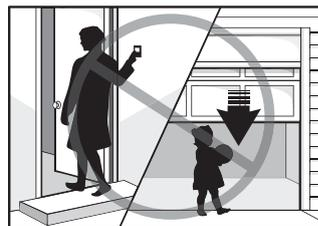
Keep the door in sight until it completely closes when using the wall-mounted push button or transmitter.
