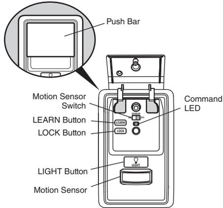
**SYNCHRONIZE THE DOOR CONTROL:** To synchronize the door control to the garage door opener, press the push bar until the garage door opener activates (it may take up to 3 presses). Test the door control by pressing the push bar; each press of the push bar will activate the garage door opener.
