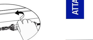
7. Remove the hook after tightening the belt tension properly.
