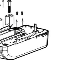
6. Detach the sprocket assembly from the rail.
