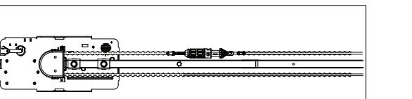
4. Tighten the turnbuckle by rotating the turnbuckle only.
