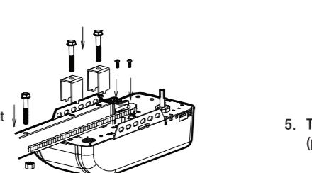
2. Insert a bolt to the stop bolt hole and secure it with nut.
