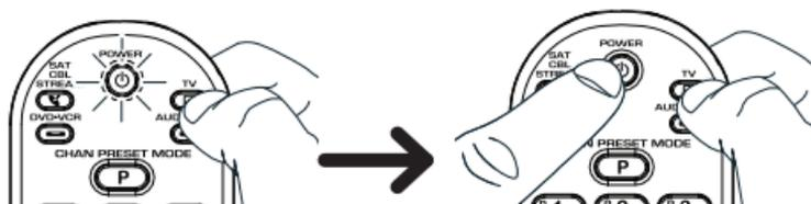
3. Wait until the remote's POWER key comes on and stays on. Then release both keys.
