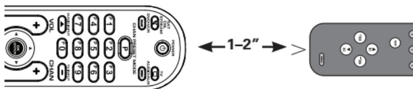
2. On the learning remote, press and hold the device key you want to use the learned function in (the POWER key turns on and remains on). While holding down the device key, use your other hand to press and hold the RECORD key (the POWER key illumination turns off).
