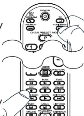
3. Wait until the POWER key turns on and stays on. Then release both keys. The remote is now in Learning mode.
