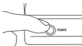
2. Press and hold the device key you want to program (the POWER key illuminates). While you're holding down the device key, use your other hand to press and hold the remote's POWER key at the same time (the POWER key turns off).
