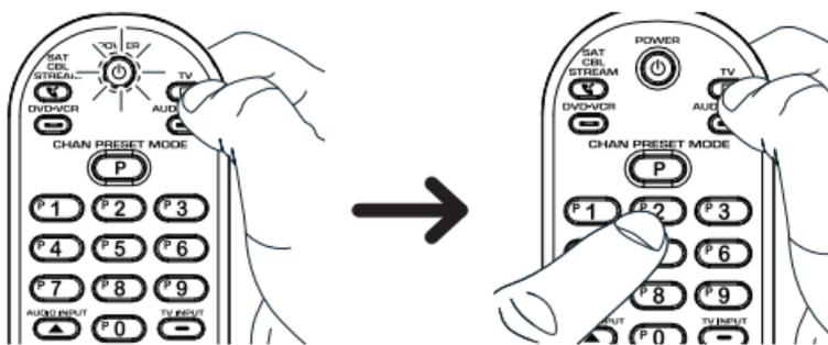
4. When you've finished entering the five-digit code, keep holding down the device key and look at the POWER key.
