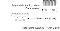
removal for cleaning, replacement or because they are out of alignment, slide the cutter back onto the black plastic oscillating head. Next, you must make sure that the cutter (small blade) and the cutting comb (large blade) are properly aligned. Line up the new or existing cutting comb with the two screw holes. Place the original screws, one in each hole, and lightly tighten with a Phillips-head screwdriver.
