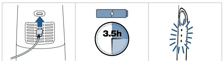
**IMPORTANT:** Always turn machine OFF before charging. Failing to do so may result in battery not fully charging.
