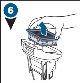
Remove the filter from the top of the dirty water tank by pulling it up.
