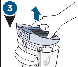
Grasp top of dirty water tank in recessed areas on each side of the filter and pull upward to remove the top of the tank.
