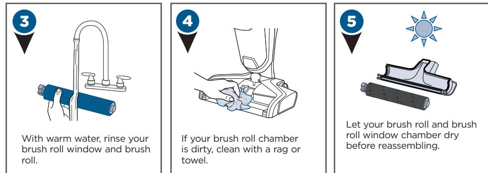
**TIP:** Running your machine with a wet brush roll will help the brush roll dry faster. The trigger should not be pressed.
