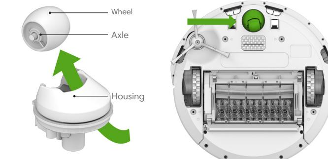
**Important:** A front wheel clogged with hair and debris could result in floor damage.
