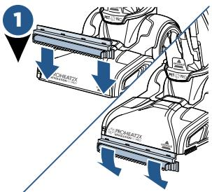
With the machine unplugged, attach the Bare Floor Tool to the bottom of the machine by lining the tool to the edge of the nozzle. Rotate down until it clicks into place.
