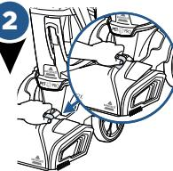
Remove the Nozzle from the foot: scoop and grip the accessory hose door. Pull up to remove the Nozzle.
