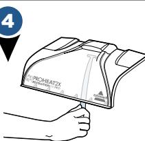
At this point, the Nozzle and Brush Roll cover can be rinsed under running water and the Nozzle Clean Out Tool can be inserted to unclog hair or debris.
