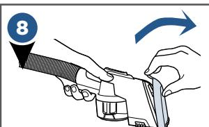
To remove any hair or trapped debris from the nozzle, first turn OFF the machine. Pull the nozzle tab away from the tool to remove and rinse under running water.
