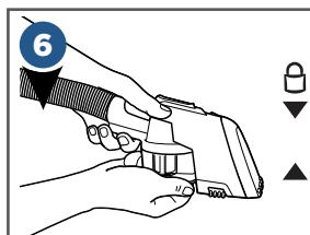
To reattach the cup, line up the cup to the tool indents, and rotate clockwise. The arrow will line up with the locked icon when secured.
