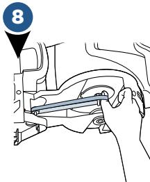
Keep it wrapped on the red pulley and adjust the machine so it is laying on its back again. Use your thumb to stretch the flat belt back to wrap around the metal axle.
