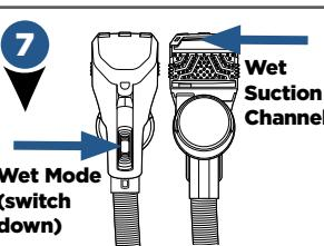
To Deep Clean, move the switch to wet mode. Press the trigger to spray your water and formula; use the top of the nozzle to extract stains and odours.
