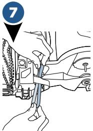
If the flat belt is broken, gently remove the belt. If it needs replacing for any reason, the gear belt should already be removed before removing the flat belt. Rotate the machine back to its side. Feed the new flat belt through the opening so that it wraps around the red pulley.
