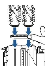
Align Brush Rolls with belt at other end. To ensure alignment, hold the end of one Brush Roll and twist. The other Brush Roll rotates with it. **Check that washers are in place.** Reassemble the belt and end cap, securing with screws you removed.
