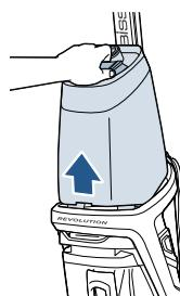
Lift the tank straight up to remove from the machine.
