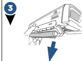
When finished, unplug the machine and remove the bare floor tool by rotating the tool up to unhook from the nozzle.
