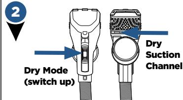
Attach the tool and select dry mode to first pick up dry debris and pet hair. The suction will be at the lower part of the tool, near the dry cup.
