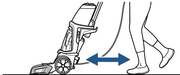
**To flush and rinse the machine:** Turn the machine ON and press the trigger for 15 seconds while making back and forth passes on a section of carpet.
