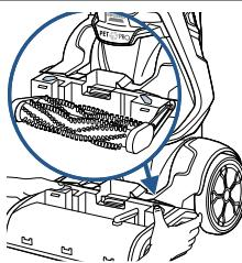
Next, remove the next layer, the Brush Roll cover, to reveal the Brush Rolls. Press on the two release buttons and lift straight up.
