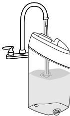
First, fill the Clean Water Tank with warm tap water and then empty it all to rinse. Then fill again with warm tap water and return the tank to the machine. Twist cap back on tightly.
