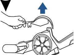
Use a flathead screwdriver and press it into the slot at the back **and then front** of the Belt Access Door. Lift to remove the door.
