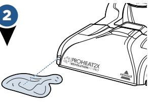
Spray will continue until you turn it off. To turn CleanShot off, press the button with your foot. The window of the button will be red and show an "O" symbol when it is off.
