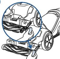
Lay the machine back down on its back. Use a Phillips-head screwdriver to remove the screw on the Brush Roll end cap.
