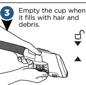
Turn OFF the machine. Hold the cup and twist counter-clockwise, line up the arrow with the unlock symbol and remove.
