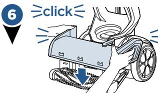
When finished, return the Brush Roll cover by pushing it straight down. You will hear a "click" from each push button when the cover is secured into place. Line up the Nozzle from the edge near the floor and rotate to snap back into place.
