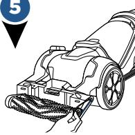
If the gear belt is broken, gently remove it. If you are replacing your Brush Rolls, gently remove the belt.
