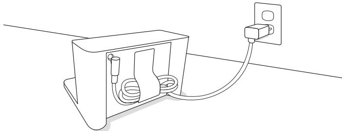
Plug the power cord into the Charging dock, then into the wall. Wrap the cord back so it won't get in the way of the robot as it comes and goes.
