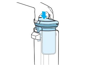
**5.** Allow tank and lid to air dry. Reinstall tank lid.
