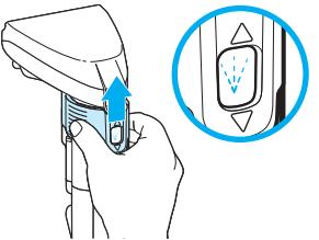
**3.** To continue cleaning with your machine, slide the tool's lever upward to return to SPRAY mode.
