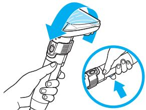
**2.** Press the trigger to activate the CLEANOUT function. Solution mixture will come through the tool and the hose.
