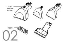
Press the cover release button on the tool and pull off tool cover. Remove the insert by pulling it off with force, if necessary.
