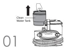
Place the spot cleaner on the ground. Lift up the clean water tank from the side of the unit.
