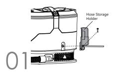
Loosen the screw pre-attached on the hose storage holder. Secure the hose storage holder onto the spot cleaner body with the screw. Tighten the screw with a cross-head screwdriver. Ensure that the screw is secured.
