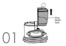
Lift up the dirty water tank from the side of the unit.
