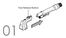
Unwrap the hose from the unit. Check to make sure the tough stain tool is connected securely
