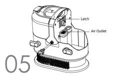
Before replacing tank back into the unit, remove any debris from the air outlet area as shown.
