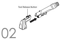
Align the tough stain tool with the end of the hose and insert it into place until you hear a 'click'.
