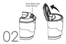
Pull the dirty water tank cover release horizontally, and open the cover.
