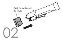
Attach the hose cleaning tool to the hose. Ensure any tools or attachments are removed.
