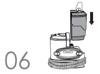
Replace the dirty water tank back into the unit, pressing down until it is locked by the latch.
