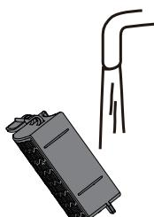
Wash with cold water only. DO NOT use detergent or soap. Allow parts to dry 24 hours before putting back into vacuum cleaner.
