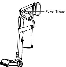
Insert the battery pack along the support rails into the battery housing. Ensure it clicks firmly into place. Press the power trigger to start the vacuum.
