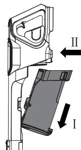
Place the clean and dry pre-filter back to the dust bin. Make sure the pre-filter is secured in place.
