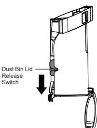
**NOTE:** For your convenience, the dust bin lid can be opened without removing the dust bin from the vacuum body. You can just slide down the dust bin lid release switch to open dust cup lid to empty the dust bin.
