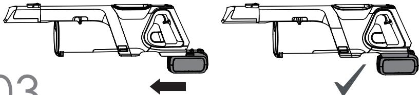
Insert the battery pack along the support rails into the battery housing. Ensure it clicks firmly into place.
