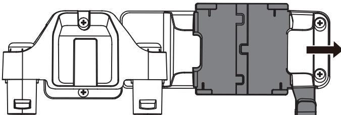
Pull out the free end of the charger bracket as shown.
