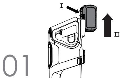
01 Press the battery release button to release the battery pack and pull the battery pack out to remove it from the hand vacuum.
