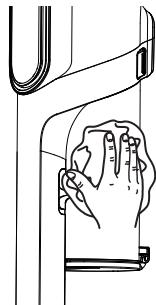
Use dry cloth to clean the outside of the unit. Do not allow any kind of liquid to enter the unit.
