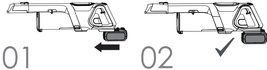
01 Align the raised rib on the battery pack with the grooves in the battery housing, and then slide the battery pack onto the hand vacuum.
