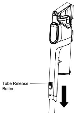
Press the bendable tube release button to remove the tube from the hand vacuum.
