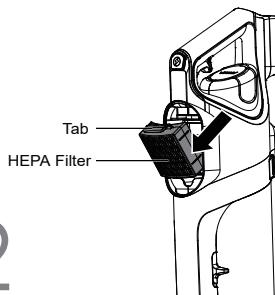
Remove the HEPA filter from vacuum cleaner by pulling the tab outward at the top of the filter.
