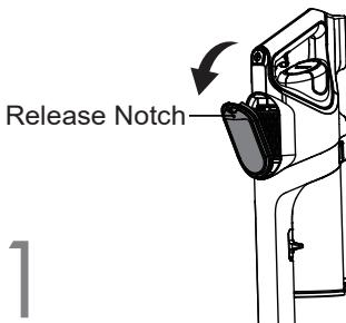
Remove the HEPA filter cover by pulling outward the release notch at the top of the cover.
