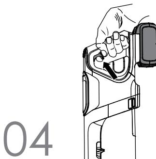
Optional: To switch the speed to HIGH speed, press the power boost button. When vacuum operates in HIGH speed, the power boost button will be lit. Press the power boost button one more time to switch back to ECO speed.
