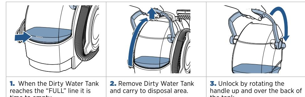
**1.** When the Dirty Water Tank reaches the "FULL" line it is time to empty.
