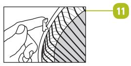
Press remaining Grille Clips onto Front Grille to securely attach Front Grille. Do not operate fan without Grille in place.
