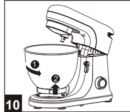
10 Remove attachment by turning the attachment counter-clockwise and pull to remove.
