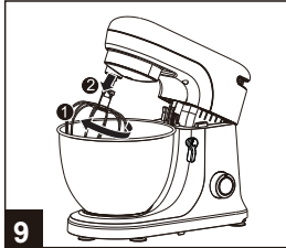
9 Remove attachment by pressing attachment upward as far as possible. Turn the attachment clockwise and pull to remove.
