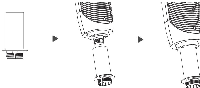
3. Attach the fan body to the base with the plastic nut.
