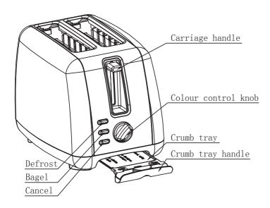
As there is manufacturing residue or oil remaining in the toaster or on the heat element, it usually emits an odour the first time it is used. It is normal and will not occur after the toaster has been used a few times. Before toasting the first slice of bread it is strongly suggested to operate the appliance following below instructions, except without bread.
