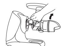
9 To disassemble, press and hold the ▲ button while turning the feed chute chamber clockwise and remove from motor base.
