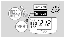
When the boiling process has completed, a melody sounds, the BOIL light turns off and the KEEP WARM light turns on.
