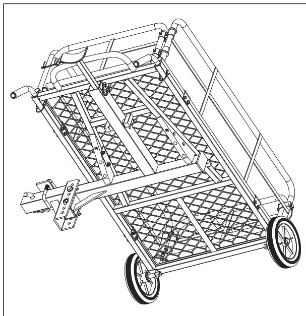
2. Roll the Carrier Platform with wheels close to the Support (B) from the curb side. Make sure the two wedge guides under the Carrier Platform (A) are between the two Tips on the Support (B). Keep the Carrier Platform (A) in tilt status, and slide up it until the end of wedge guides sit right on the Square Beam of the Support (B), check and make sure two Latch A are locked down the two Tips.
