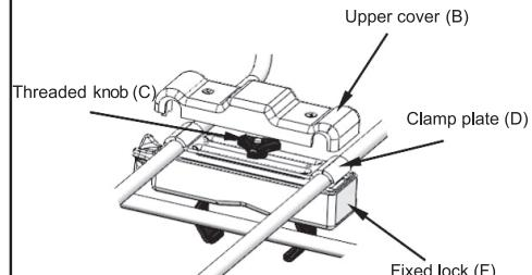
By placing the fixed lock (F) under the cross bar, clamping the splint (D) on the cross bar and sliding over the fixed lock, the square neck bolt of the fixed lock passes through the splint and is tightened and fixed with the thread knob (C). Check the overall suitability and tightness of all parts.
