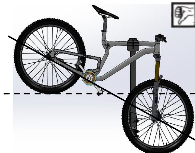
**Not loading the bikes properly can result in damage, injuries or death!**
