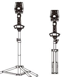
**Warning:** Be careful not to get your hands crushed when extending the tripod legs. Place the tripod on a stable, flat surface.
