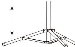
To adjust the tripod height, loosen the top tripod locking knob on the top of the tripod, adjust to the desired height, then tighten the tripod locking knob.
